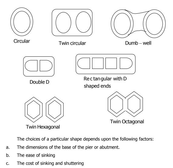
d. The vertical and horizontal forces acting on the well
