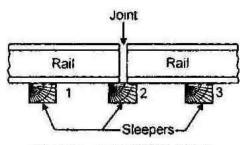
Fig. Supported Rail Joints
