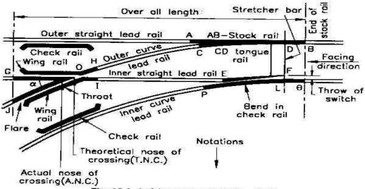
Fig. 16.1. Left hand turnout (Split switch).
