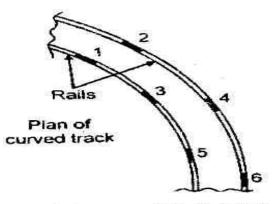
Fig. Staggered Rail Joint
